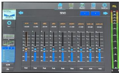
Digital channel signals are routed to the output page
